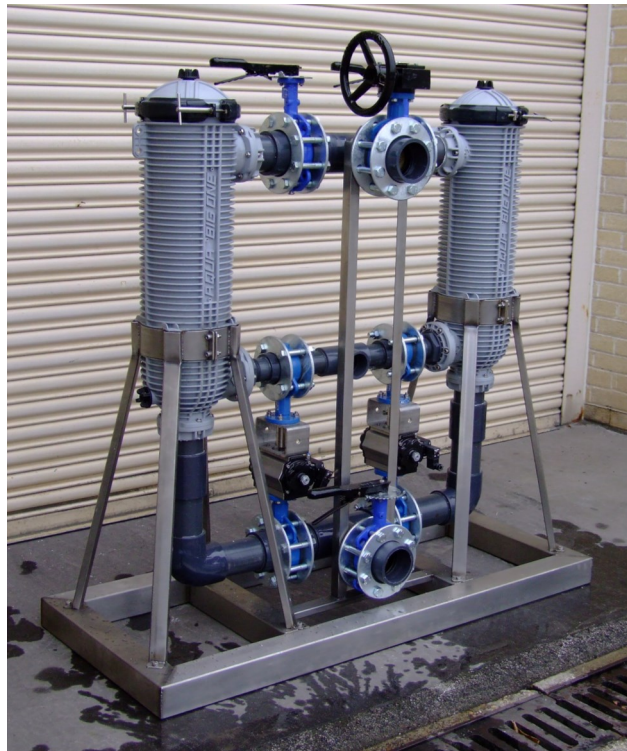
TWO POD FILTER UNIT WITH 3" INLET AND RETURN. BACKWASH PORT 2".
